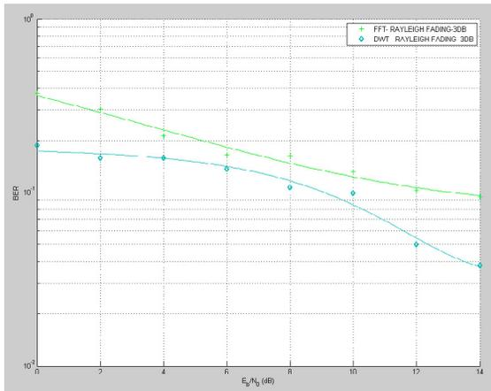
**Fig. 6.** BER values with relations  $E_b/N_0$  from 1-14dB for RAYLEIGH channels.
