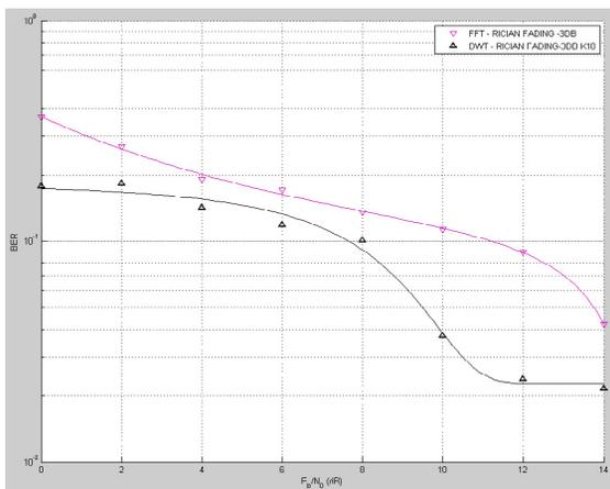
**Fig. 7.** BER values with relations  $E_b/N_0$  from 1-14dB for RICIAN channels
