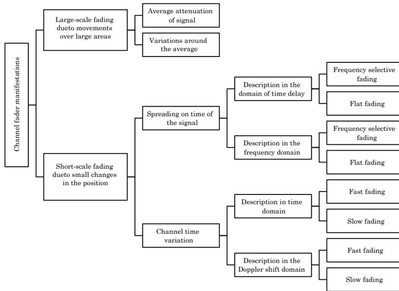
**Fig. 1.** Fading types in a wireless channel.
