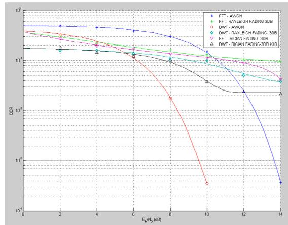
**Fig. 8.** BER values with relations  $E_b/N_0$  from 1-14dB for AWGN, RAYLEIGH, and RICIAN channels.
