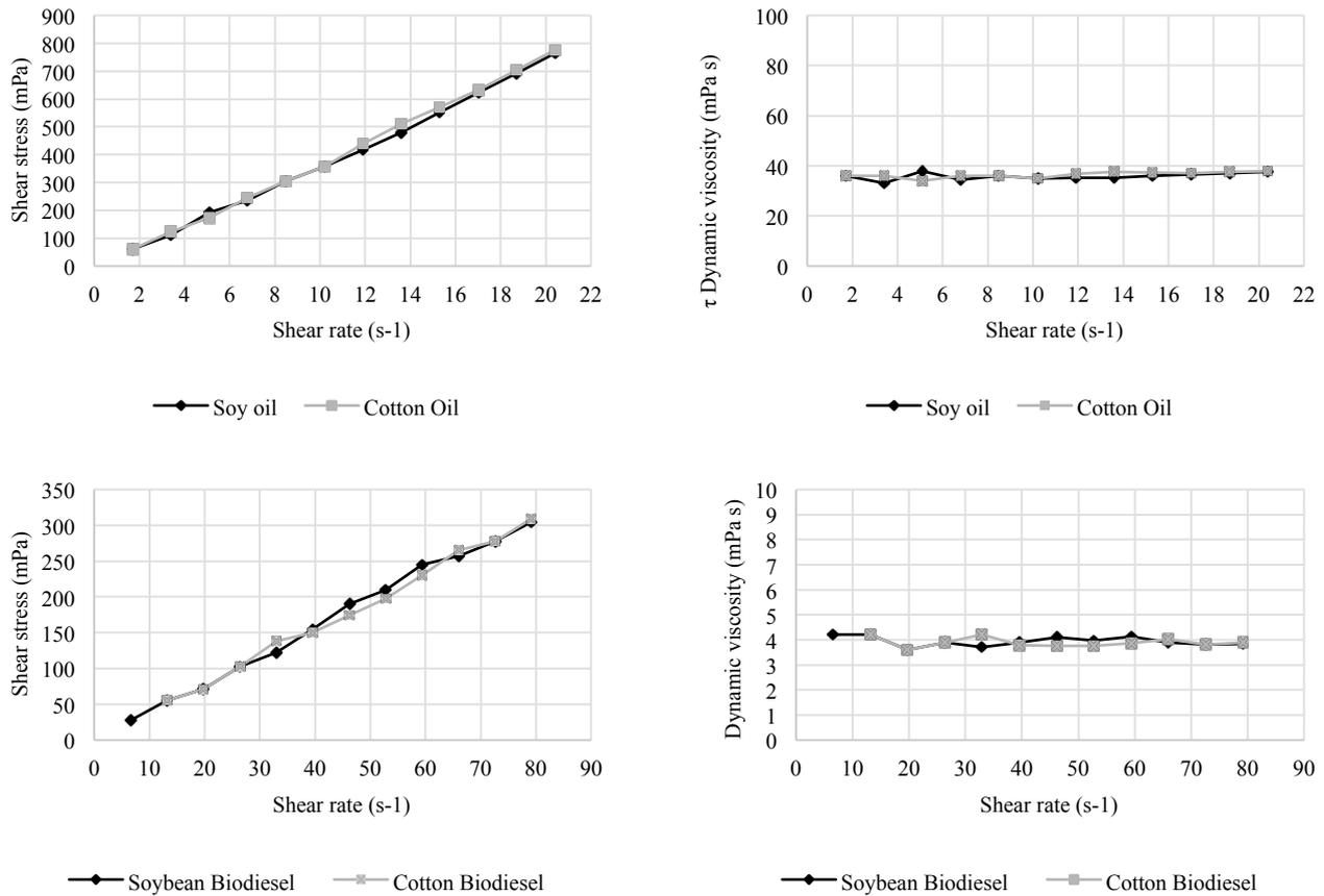
Fig. 2. Characteristic graph of Newtonian fluids made for soybean and cotton oils and soybean and cotton biodiesel.
