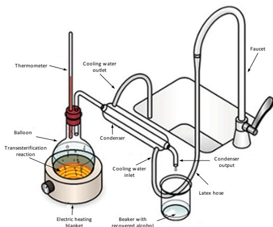
**Fig. 1.** Scheme of the system for the synthesis of biodiesel.
