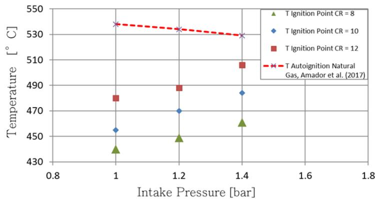
Figure 2: Comparative modeled temperature at the ignition point and Auto-ignition temperature of Natural Gas
