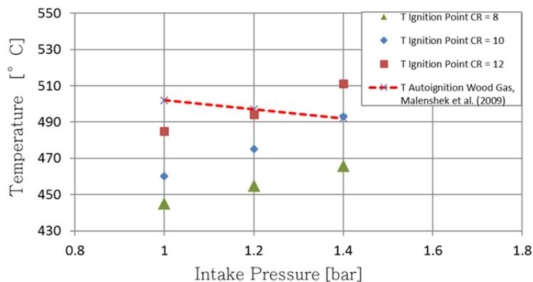
Figure 3: Comparative modeled temperature at the ignition point and Auto-ignition temperature of Wood Gas
