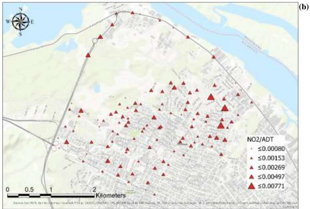
**Figure 4 a,b.** Average daily traffic - ADT (a) and relation between NO<sub>2</sub> concentration/ADT (b)
