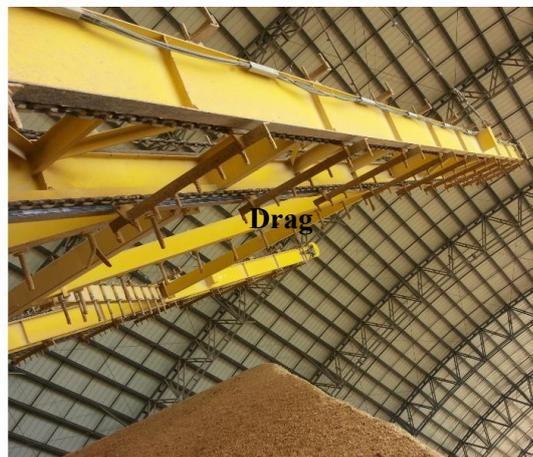
**Figure 1.** Drag system in the limestone reclaimer
