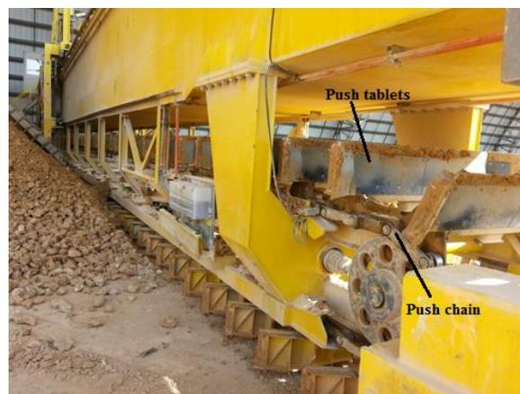
**Figure 2.** Push device in the limestone reclaimer.
