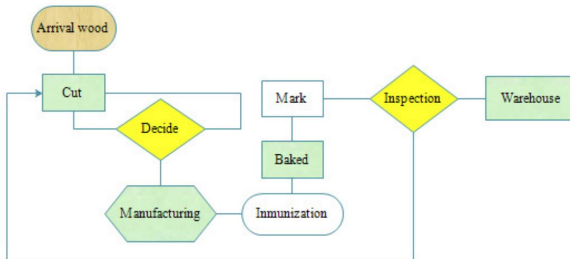
Fig. 2. Flow chart of wood stowage manufacturing.
