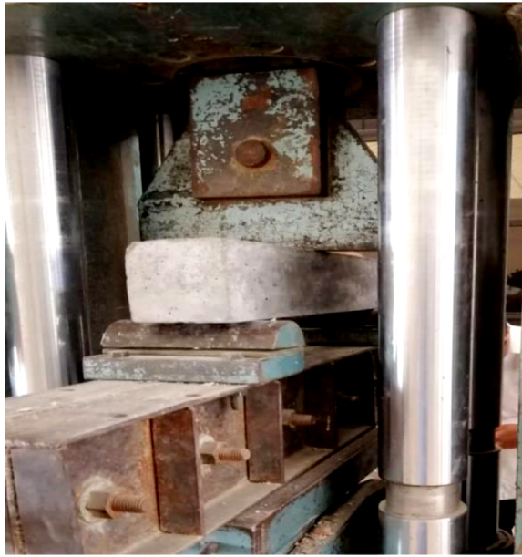
Fig. 3. Flexural Strength Test.
