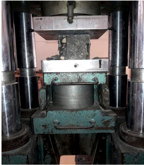
Fig. 1. Compressive Strength Test.
