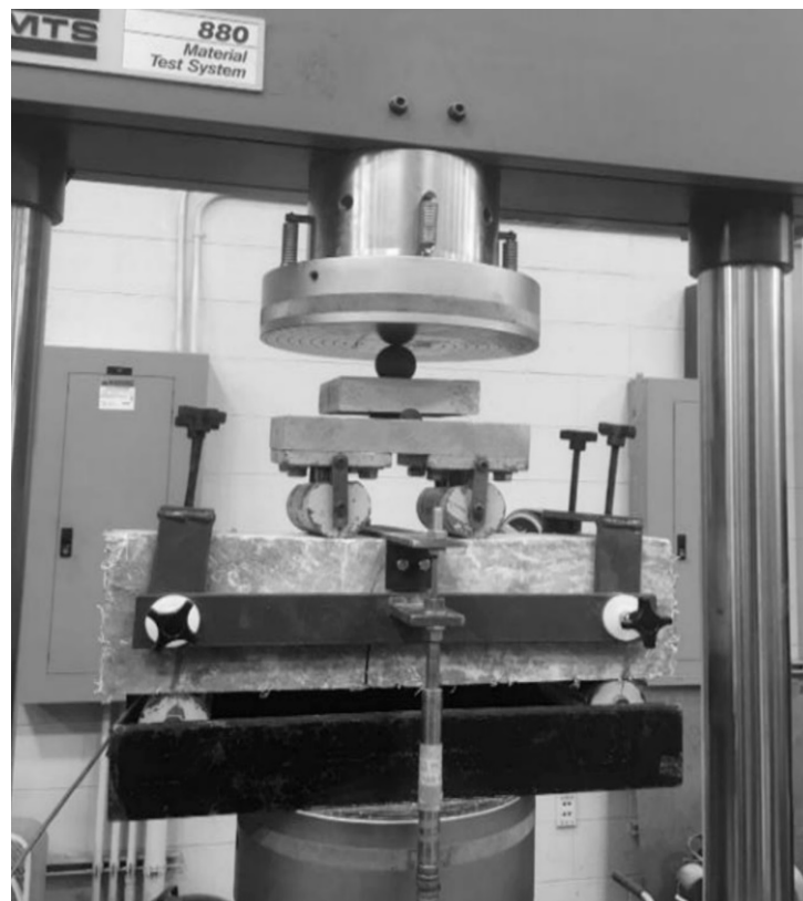
Figure 2. Illustration of 4-point bending testing for UHPC prisms.
