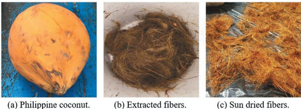
Figure 1. Coconut fiber extraction untreated. (a) Philippine coconut; (b) Extracted fibers; (c) Sun-dried fibers.
